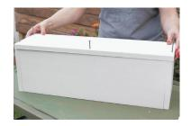
Create the borders along the top of the planter. Use three to four 2" screws to connect the long tops to the long sides and two 2" screws to join the short tops to the short sides. Place the screws .5 - 1" in from the ends and in the center of the top pieces.
