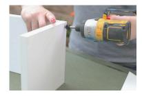
Assemble the sides to the base, starting with the short sides. Lay the base on a flat surface and use four 2" screws to connect short sides A (8x7 1/4") to the shorter sides of the base. Then use five 2" screws to join long sides B (8x24") to the long sides of the base (one per corner and in the middle).
